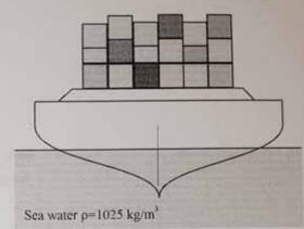
$$\sqrt{DISP} = \frac{W}{V_W} = \frac{26500 \times 10^3 \,\text{N}}{1025 \,\text{kg}_{\text{m}^3} (9.81 \,\text{m/s}^2)} = 2635 \,\text{m}^3$$
