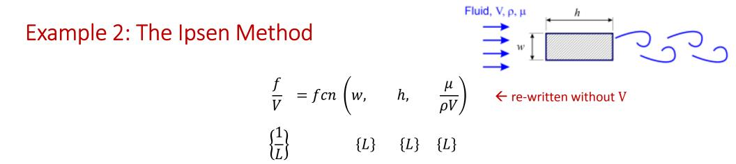
• Now we pick RHS variable that contains {L}, w. This will be the characteristic dimension. We use w to eliminate {L} in the terms that contain the dimension of length.
