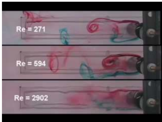
Vortex shedding behind a cylinder.
