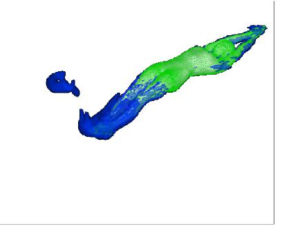
Computation Fluid Dynamics Simulation a Swimmer. A 3-D unsteady flow with moving boundaries.
