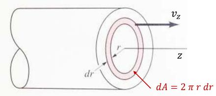
• We can integrate this velocity field to get the volume flow rate:
