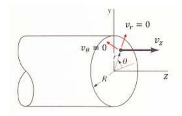
$$\rho \left(\frac{\partial v_z}{\partial t} + v_r \frac{\partial v_z}{\partial r} + \frac{1}{r} v_{\theta} \frac{\partial v_z}{\partial \theta} + v_z \frac{\partial v_z}{\partial z}\right) = -\frac{\partial p}{\partial z} + \mu \left\{\frac{1}{r} \frac{\partial}{\partial r} \left(r \frac{\partial v_z}{\partial r}\right) + \frac{1}{r^2} \frac{\partial^2 v_z}{\partial \theta^2} + \frac{\partial^2 v_z}{\partial z^2}\right\}$$
