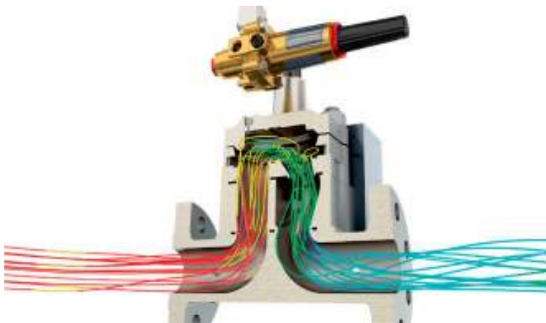
Analysis of pressure losses across a valve
