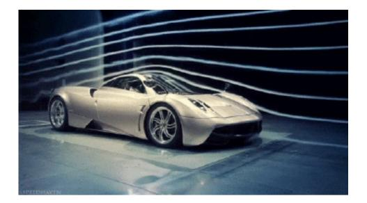
Streaklines (streamlines) over a high performance car. The Bernoulli equation would apply for this flow, except very near the surface. Source: http://6speedhaven.tumblr.com/post/25448453293
