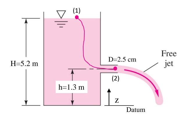
We have:  $V_2 = 8.75 \frac{m}{s}$ Thus, the discharge flow rate is:  $Q = V_2 A_2 = V_2 \pi \frac{D_2^2}{4} = \frac{8.75m}{s} \pi \frac{(0.025m)^2}{4} = 0.00429 \frac{m^3}{s} = 4.29 l/s$ (Will the actual flow likely be higher or lower? Why?) Ans.
