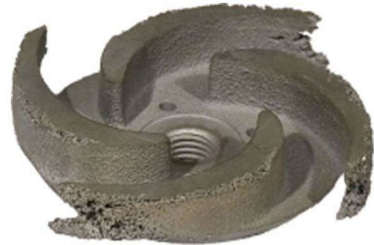
Damaged pump impeller
